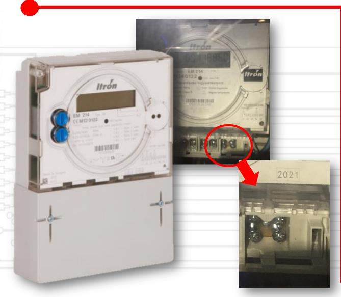
The 20/21 terminal is at the right corner of the electric meter, as shown, to which the iMachine pulse counter input can be attached with 2 wires.
