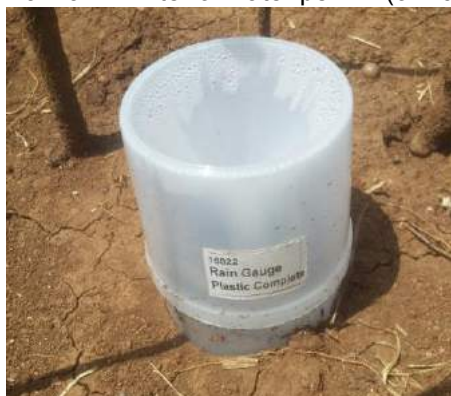
Plate 6: Rain gauge was installed at the trial site
