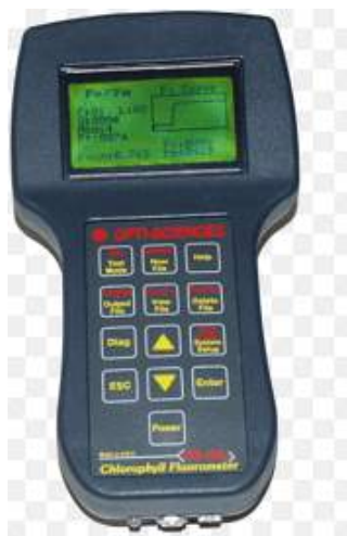
Photo 6. fluorimeter OPTI-SCIENCES OS30p+
